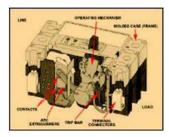
**Figure 3:** Cutaway of a molded case circuit breaker showing numerous infrared inspection points (courtesy of Cutler-Hammer University).
